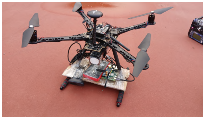
Figure 2: The prototype UAV with onboard Raspberry Pi 5, cellular modem and NB-IoT modules.
